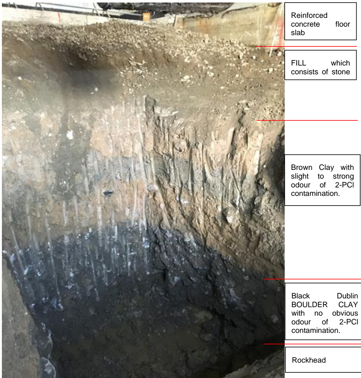
Lithology sequence present within MWPB at Arch Chemicals site. Bedrock encountered in the range of 5.5mbgl to 6.25mbgl.
