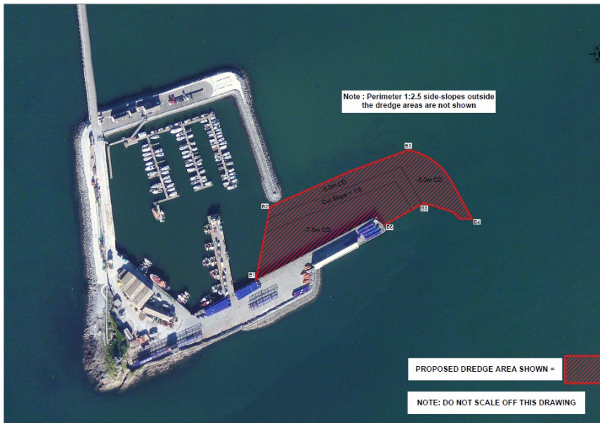
Figure 2 Dredging areas in Fenit Harbour, image from Dutch Dredging Method Statement.
