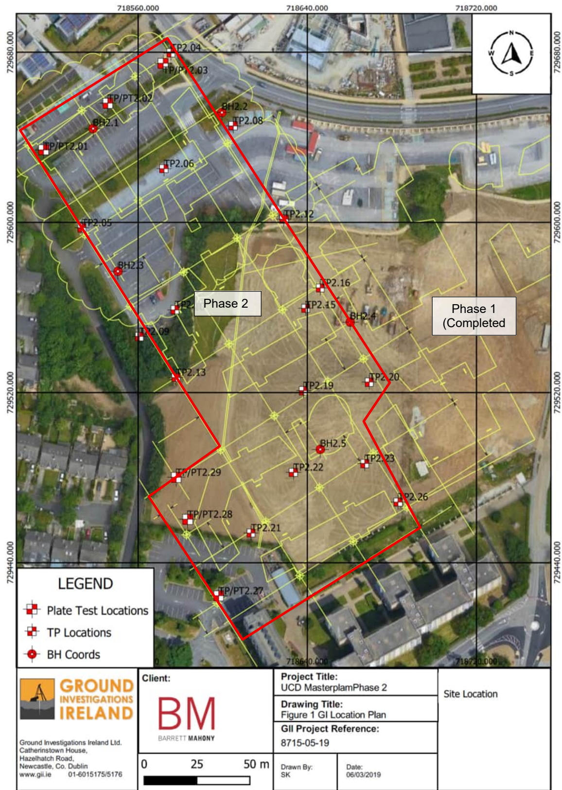
Figure 2.3 – Site Investigation Location Plan and Building Overlay
