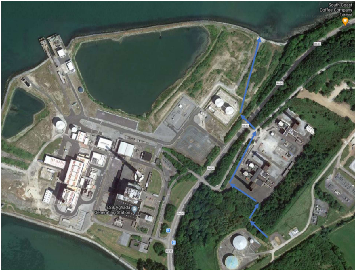
Figure 4 Satellite view of Aghada Generating Station showing the proposed surface water connection to the existing surface water network. From here, surface water is conveyed to the outfall at the SW12 water emissions point in Cork Harbour via the existing CT'S interceptor.
