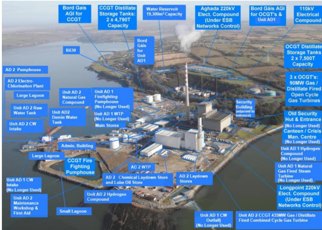
Figure 2-2 Existing Power Station Layout
