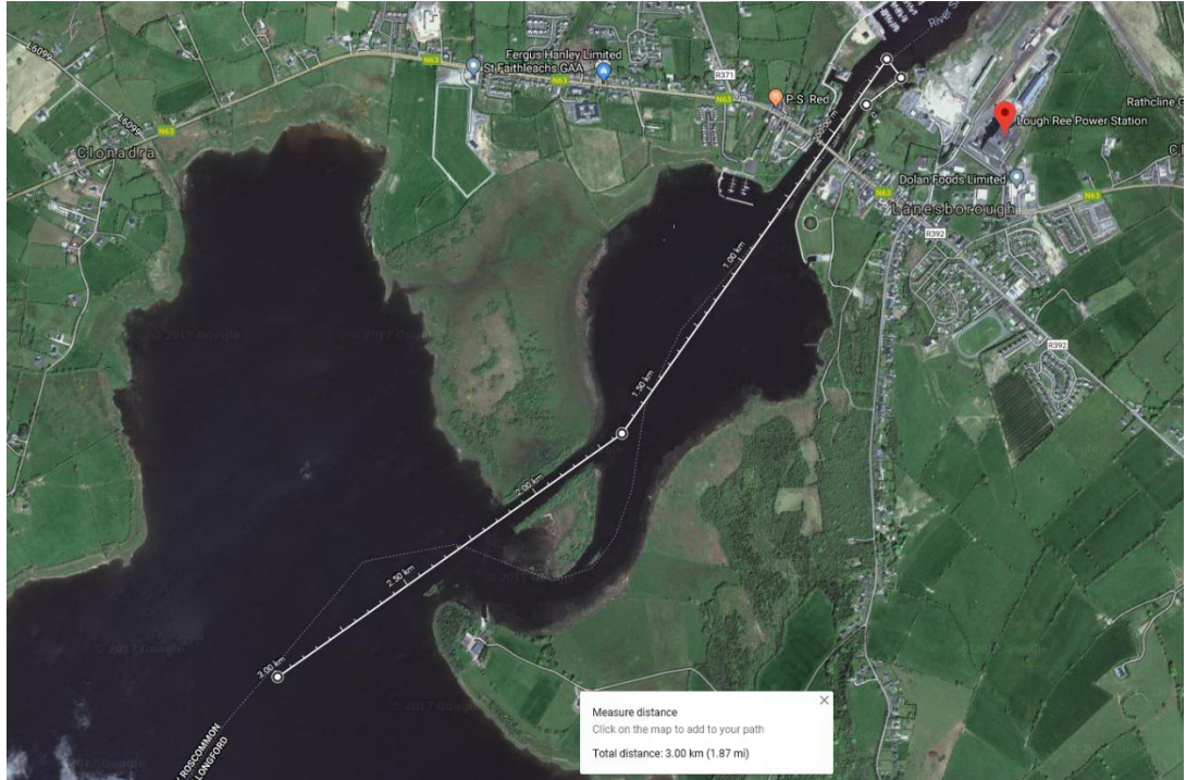
Figure 3-5: CW Connections to Lough Ree with Pump and Mixing Pipe Approximately 3000m of new underwater Piping, and a new Pump House or annex
