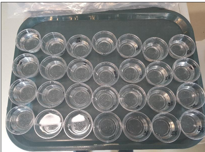
Plate 23 Daphnia magna 48 h EC 50 test
