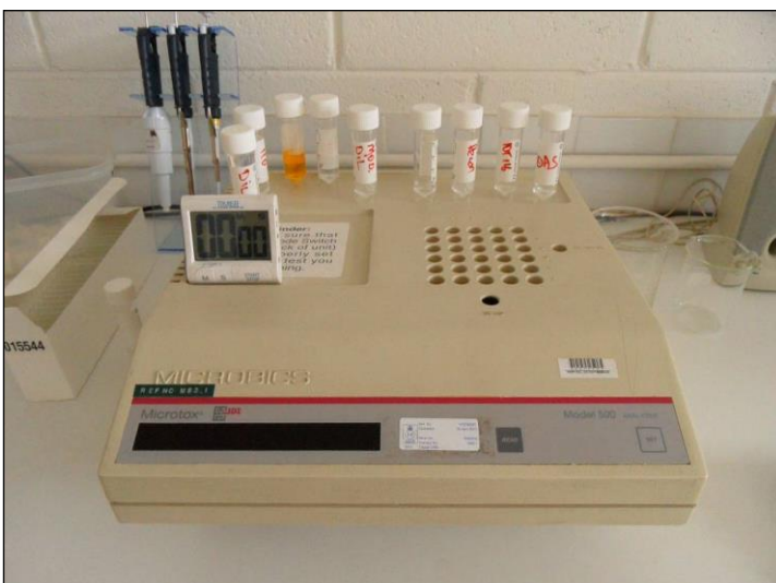
Plate 24 Temperature controlled photometer apparatus used to test for bioluminescence of Vibrio fischeri in the 30 min EC 50 test.
