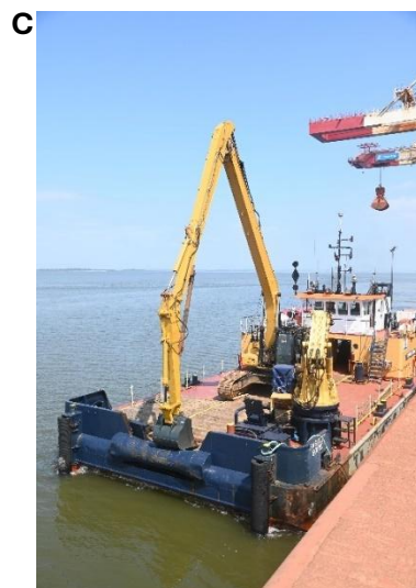
Figure 3. Ploughing operations at the Aughinish Alumina marine terminal jetty. (A) the bed levelling unit is raised here, this is used for ploughing operations, (B) the Fastnet Sound carrying out ploughing operations, the bed levelling unit is dropped to the sea bed (C) & (D) excavating operations being conducted from the Fastnet Sound by the long arm tracking machine.
