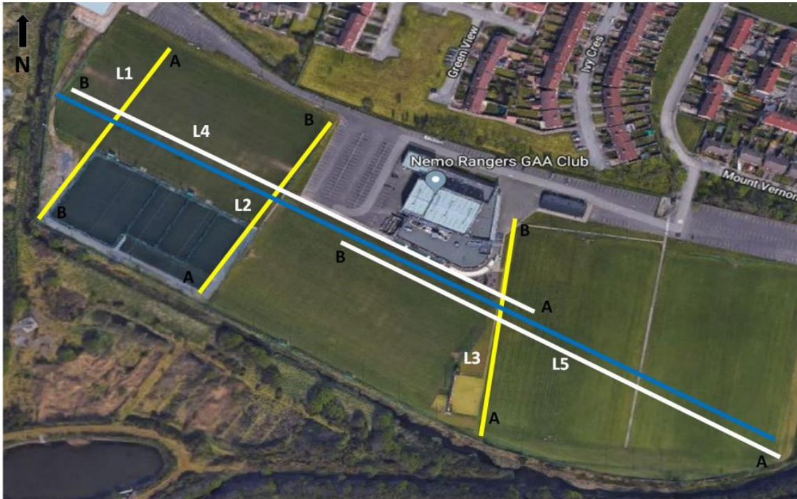
Geophysical Survey Lines Conducted on the Nemo Rangers Grounds (Profile Lines 1-5)
