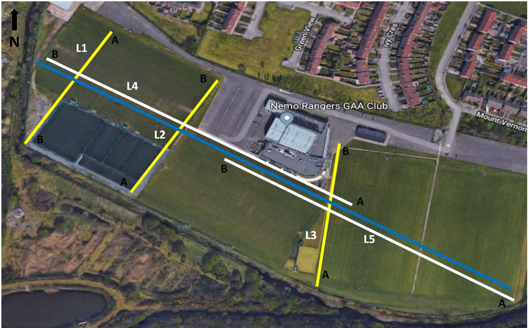
Geophysical Survey Lines Conducted on the Nemo Rangers Grounds (Profile Lines 1-5)
