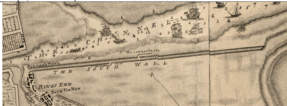
Detail from Rocque 1757, showing the South Wall as constructed prior to its completion in 1759. Note the two slipways attendant to the wall, referenced ADCO 04 and DCIHR
