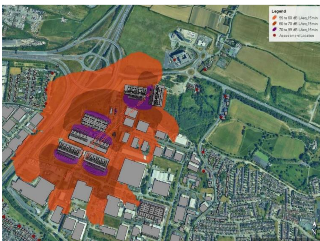
Figure 6.3: Predicted noise levels when generators are in operation (Scenario B) (From Attachment-7-1-3-2-Noise Emissions Impact 2, January 2022).
