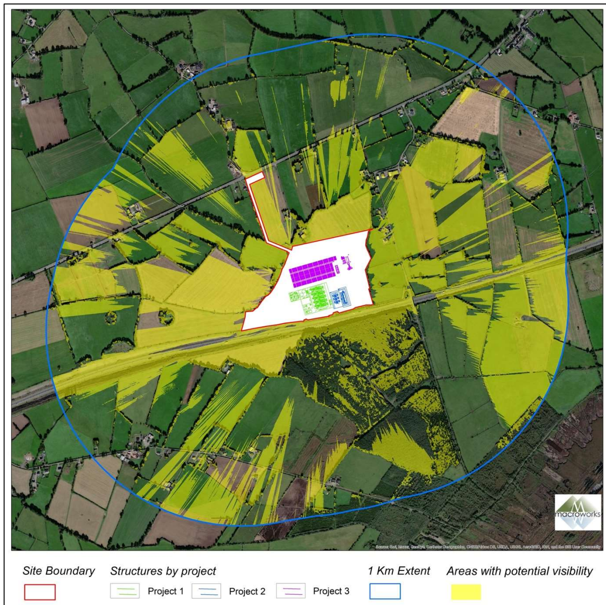
Figure 11.7 Digital Surface Model (DSM) based ZTV map accounting for screening by surface elements such as hedgerows and trees lines.
