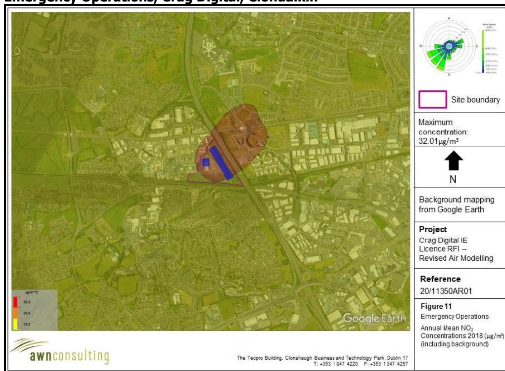
Figure 6.2: Annual Mean NO 2 Concentrations (including background), Emergency Operations, Crag Digital, Clondalkin
